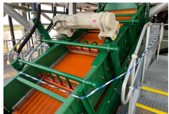
Figure 8: MSP - 30kV Coronastat Electro-static separators
