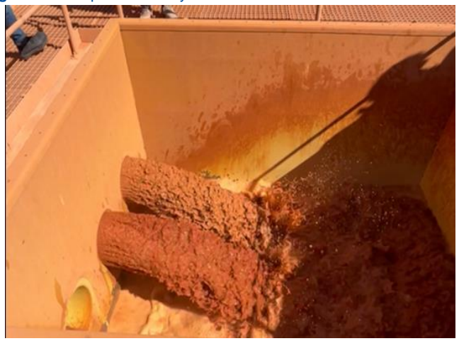
Figure 5: Receipt of ore slurry into the WCP
