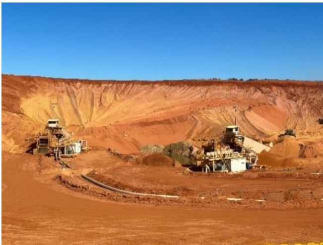
Figure 4: Pipework from the mining area into the Wet Concentrate Plant
